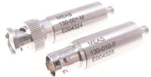
The **Model 130 series** are remote in-line charge converters designed to be used with piezoelectric accelerometers. The low noise charge converters feature three fixed gain options that convert the high impedance charge output from the accelerometer to a low impedance voltage output. The model 130 series features broad bandwidth to 30kHz and 10Vpeak linear output. The units are powered by a constant current of 4 to 20mA.
