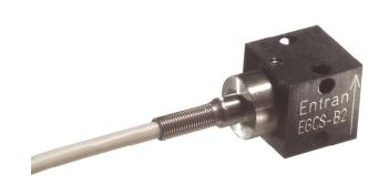
The Model EGCS accelerometers combine a damping ratio of 0.7 (Nominal) with built-in overrange stops that are set to protect the unit against 10,000g shocks. This is ideal for applications which may experience rough handling or in situations where the accelerometer must survive a high initial overload in order to make a low g measurement. These units feature a Wheatsone Bridge output with compensated temperature range of 20 to 80 °C.
