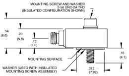
STANDARD TOLERANCE INCHES (MILLIMETERS) .XX = +/- .02 (.X = +/- .5) .XXX = +/- .010 (.XX = +/- .25)
